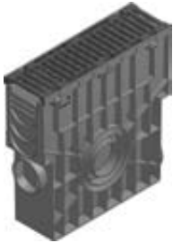
Trash box with plastic bucket, with ductile iron grating, black, SW 10 mm, class E 600, 4-fold bolted
